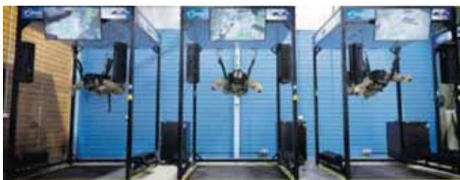
Soldiers use the J3Seven Raptor jump simulators at the ADF Parachuting School to practise a freefall parachute jump. Photos: Pte Nicholas Marquis
