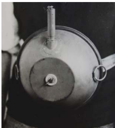
British scientist wearing an early version of the Limpet mine on a keeper plate in the position used by a swimmer. Source: UK National Archives.
