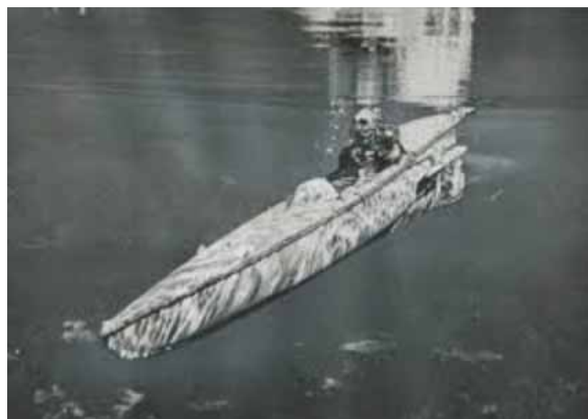
Photo 1. Motorised Submersible Canoes (MSC), commonly referred to as 'the Sleeping Beauty' Source: AWM
